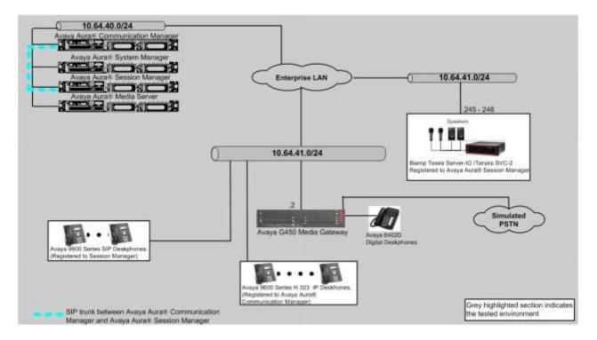
Figure 1: Test Configuration of Biamp Tesira SVC-2
